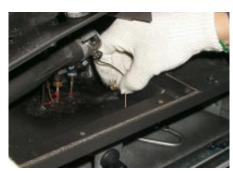
Note: when installing the burner assembly be sure to slide the aeration adjustment wire through the hole in the base of the burner tray.
